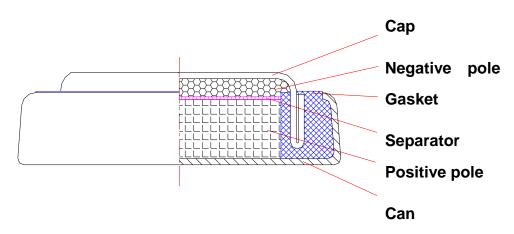
The material of the battery case is made of **stainless steel SUS 304.** There is **no** surface finishing made on the battery case material.
